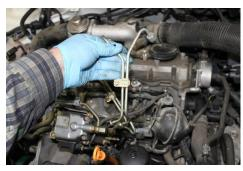
Remove the two fuel pipes and set aside in a CLEAN area.
