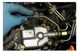
Remove the fuel return line from the pump, use a Miti-Vac to suction out air inside the pump. This requires about 25" hg for about 2-3 minutes. Once you have fuel coming from the top of the pump the evacuation is complete. Reconnect the fitting and install the clamp.
