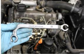
Cut the fuel return lines, these will be discarded after injector removal. Get your Hazet 4560 injector Removal wrench.
