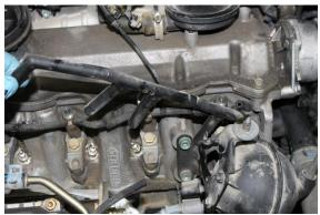
Lift up, and be careful not to bend the harness, lay over and out of the way near air-box.
