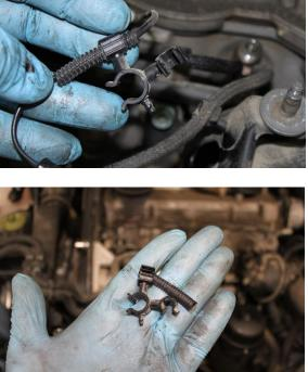
Remove and keep the wire support and protective cover for shielded wire. The support is removed by using a pick to disconnect the click lock fold over clasp.
