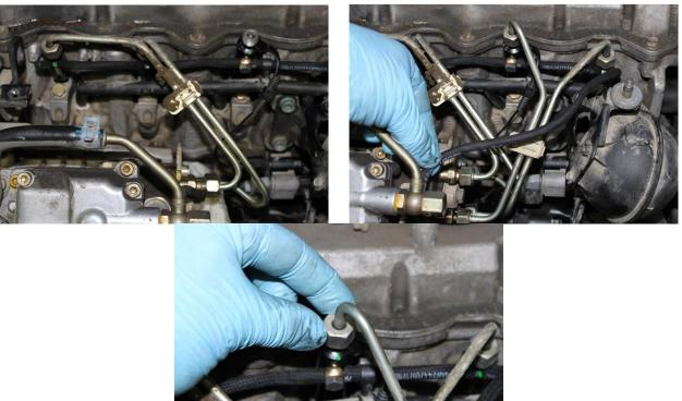
Reconnect all the lines, DO NOT over tighten, bottom the nut and add 1/8<sup>th</sup> of a turn. Leave ONLY the #3 fitting on top of the injector loose, this is to allow an air purge for the needle lift sensor when starting the first time.
