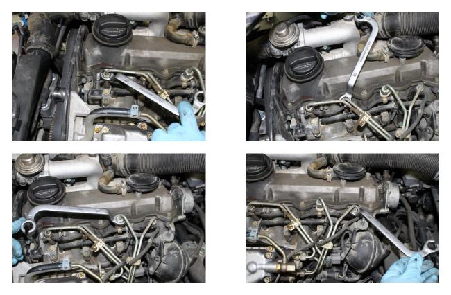
Break loose and completely loosen the (4) fittings at each of the injectors. Note that there is not (or should not be) very much torque on these.
