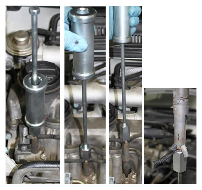
Attach the extractor firmly onto the injector threads, with multiple rapid forceful blows, extract the injector up and out of each of the bores. You are breaking the carbon loose from around the nozzle.
