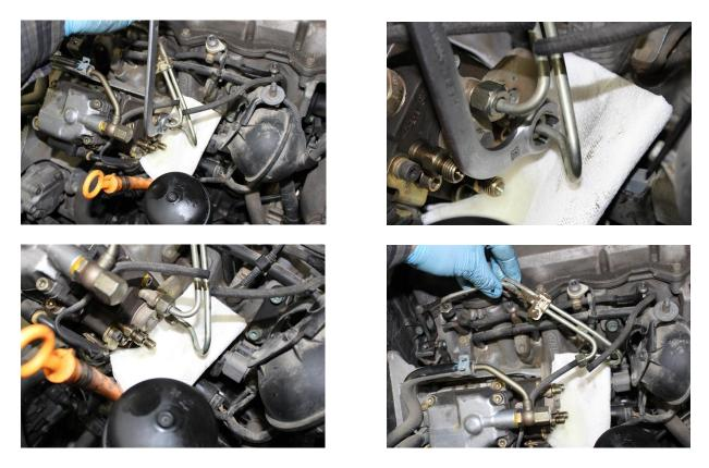
Break loose the two rear fittings and loosen. Place some paper towel underneath to catch fuel that will drip from the fittings.
