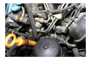
Break loose and completely loosen the two front fittings on the injection pump.
