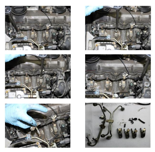
Loosen and remove the four bolts and injector clamps, be careful not to lose the special washer that is under each of the bolts. Keep each fork clamp with its respective position (not critical). You can clean the bolt threads with a wire wheel or wire brush and apply moly disulfide grease to the ball pivot under each fork clamp (this can be done when the injectors come back).
