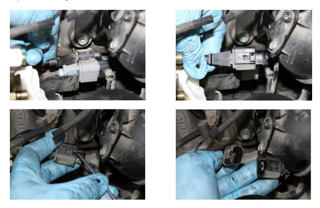
Remove #3 connector, depress tab with pick and disconnect (2003 connector pictured – Black; 2002 and earlier models use a brown "Square" connector).
