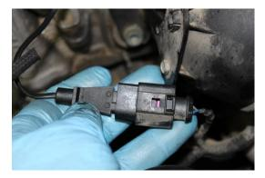
Reconnect the glow plug harness, connect the new fuel return lines. DO NOT re-use the return line, this will leak causing a fire hazard. The line has a shrink characteristic that seals it to the nipples. Always use new return line that comes in our kits.
